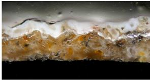
Nanocomp MM12 doesn't provide own roughness and insulation effect. It is applied thinly on standard base coatings for aluminium permanent mould casting. The MM12 coat should only be 5-15  $\mu$ m. Consumption is very low.
